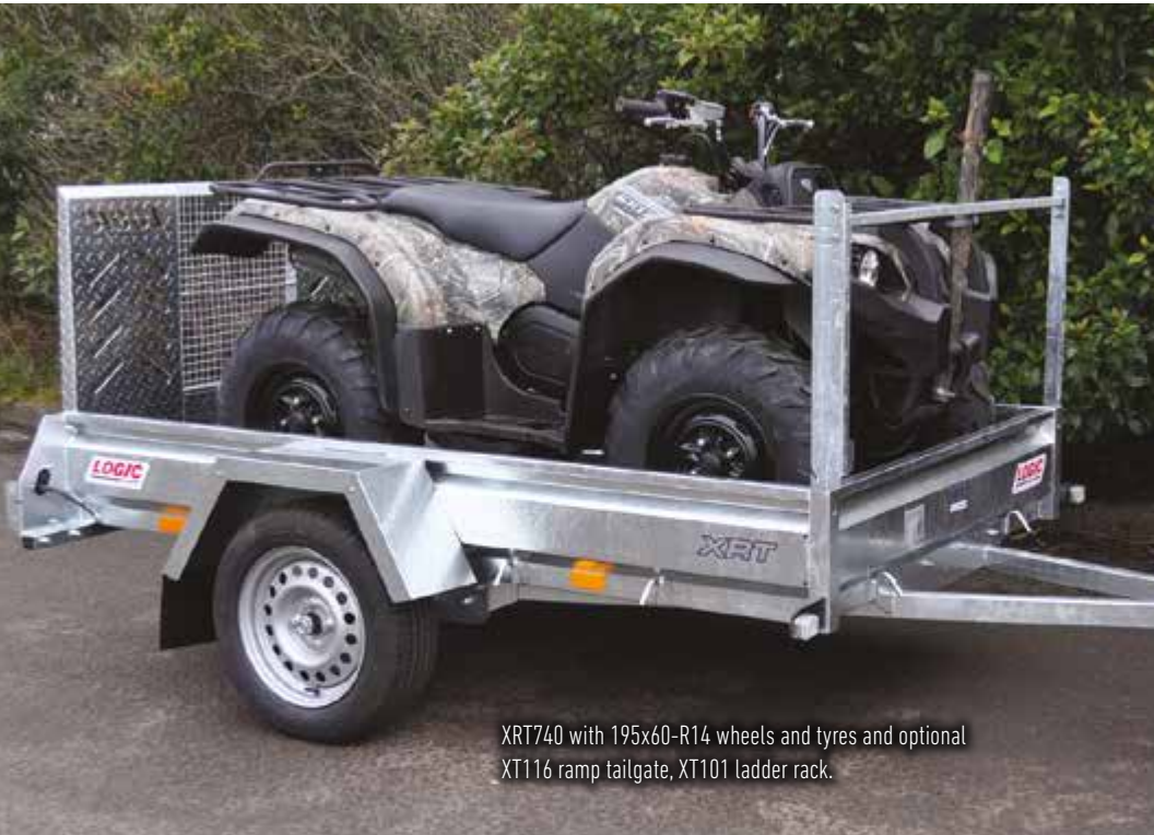
1 Optional XT116 metal loading ramp/tailgate, for loading ATVs, garden machinery, etc.
