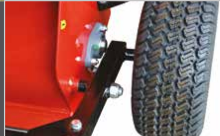
Wide rear castor wheels ensure specialist grassed surfaces are not damaged.
