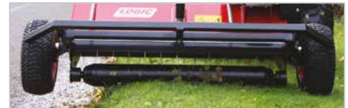
The full width anti-scalping roller (above) protects the sward from scalping and allows cutting over kerbs.
