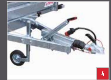
4 Overrun brakes with safety breakaway cable, handbrake and jockey wheel.
