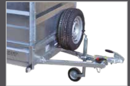
Other options include a spare wheel with WB103 mounting bracket and RT710-01 jockey wheel.
