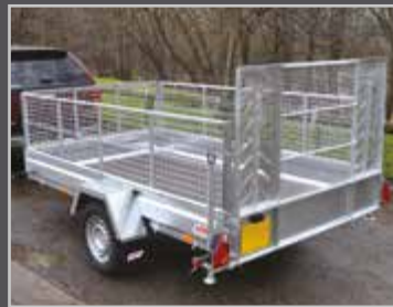
VT726 seen here with optional VT202 mesh extension sides and VT101 mesh headboard to 900mm high.
