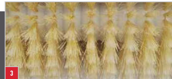
The unique nature of this Logic patented brush is fundamental to the success of the system. It is a mixture of absorbent natural fibres and synthetic fibres in interlocking rings of bristles mounted on a central shaft with a slight gap between each of them to allow plants to 'comb' through, delivering a high dose of chemical in one pass.
