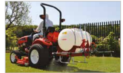
Perfect for small tractors with 'Cat 1' linkages like this compact tractor mower unit. The skid unit sets the sprayer at a good height for dismantling and storage.
