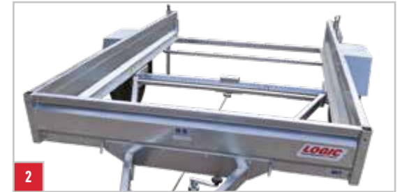
2 Monoque construction with 'A' frame drawbar, Al-Ko suspension, one piece axle (1300kg) featuring rubber progressive action with excellent dampening. All protected with hot dipped galvanising for long life.
